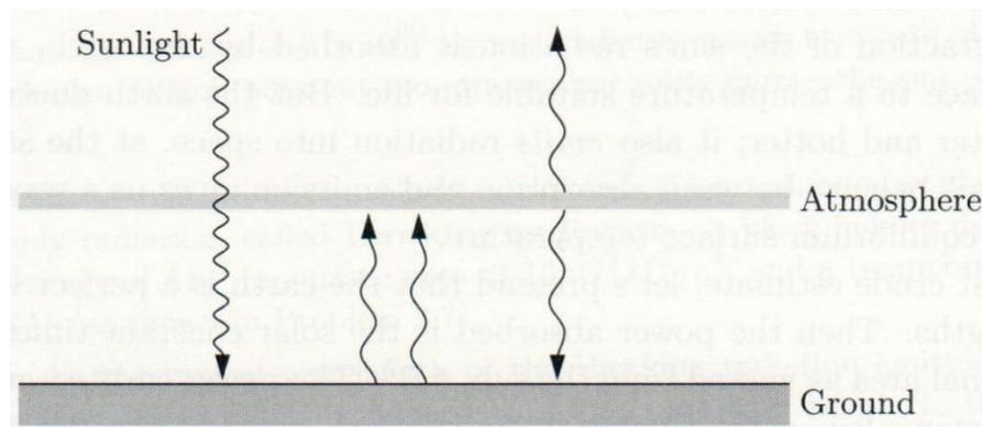
“Earth’s atmosphere is mostly transparent to incoming sunlight, but opaque to the infrared light radiated upward by earth’s surface. If we model the atmosphere as a single layer, then equilibrium requires that earth’s surface receive as much energy from the atmosphere as from the sun.”
